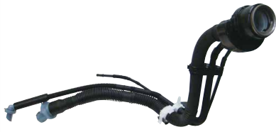
Plastic fuel filler pipes
