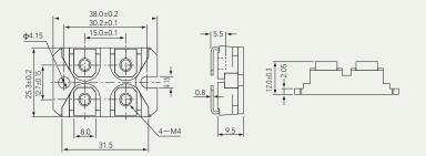
The mounting torque capability is particularly good with a value of 1,5 Nm using a M4 type of screw.
